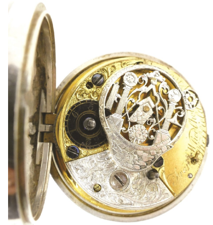
Inside the Francis Wheelhouse masonic pocket watch showing the finely fretted and engraved watch cock
